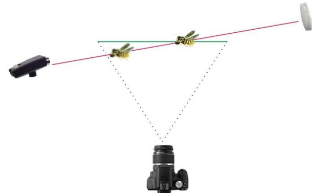
Figure 17: The plane of focus intersects the light beam
