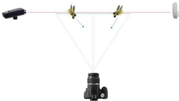
Figure 16: Plane of focus is parallel to the IR-beam
