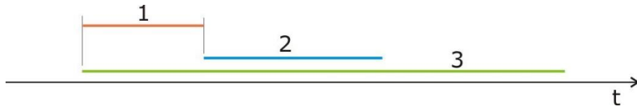
Figure 18: Time-sets of a step: 1 - delay time, 2 - ON-time, 3 - step duration time
